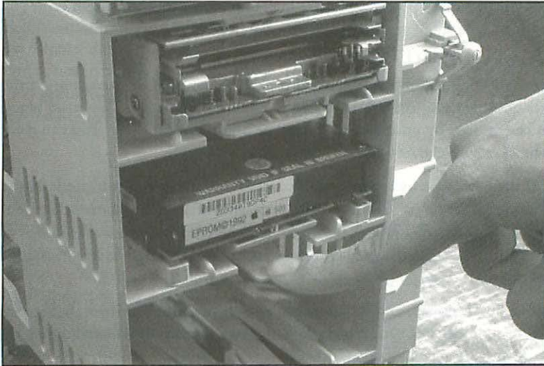
Figure 6.52 In the Quadra 840AV, press the clip and slide the drive forward.
